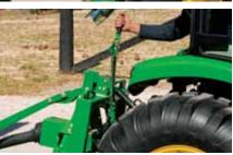
2) Once you're connected and the unit is in place, there's an even easier way to automatically hook up PTO-driven attachments. The iMatch AutoHitch is the answer. To hook up the drive shaft to the secure unit, just rotate the handle, turn and pull AutoHitch lever.
