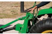
1) To quickly change implements with the iMatch Quik-Hitch, you simply back in, hydraulically lift the unit and secure the latches.
